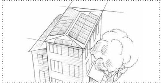
*Does your roof face in different directions? Here too, a feed-in system comprising individual inverters is the solution: Uneven irradiation conditions may even be of advantage because energy can be consumed more efficiently and throughout the day.*
