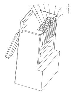
Illustration 6.2 RJ-45 Pinout Detail for Ethernet
