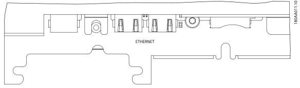
Illustration 6.1 Auxiliary Interfaces (Cutout of Inverter Installation Compartment)
