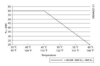
Illustration 2.7 Derating as Function of Internal Overtemperature
