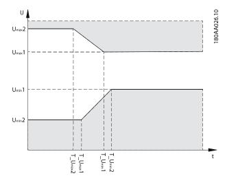
Illustration 2.11 Overvoltage and Undervoltage Disconnect
