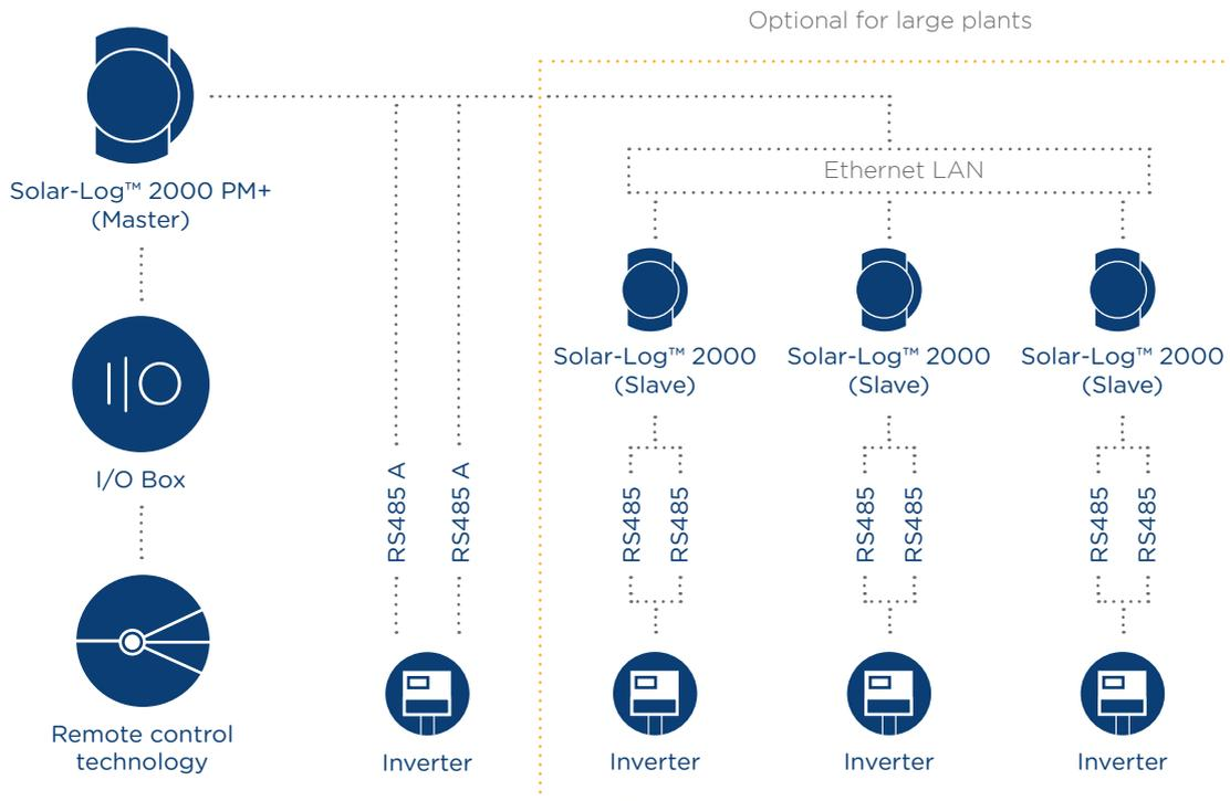
The grid operator's signals are received by the Solar Log2000 PM+ (master) and distributed to the connected inverters via the Solar-Log 2000 (slaves). The master can be connected to up to nine slaves in this setup. Linking the Solar-Logs together over the network helps to implement complex requirements (several plant parts, feeding points and inverters from many manufacturers).
