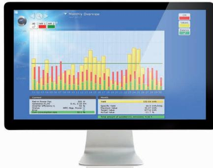
Monthly overview: Using the performance ratio graphic allows for a comparison of the potential yields, as measured by the irradiation sensors and actual yield.
